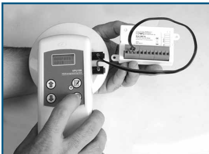
Figure 34 - Addressing modules using a VPU100
