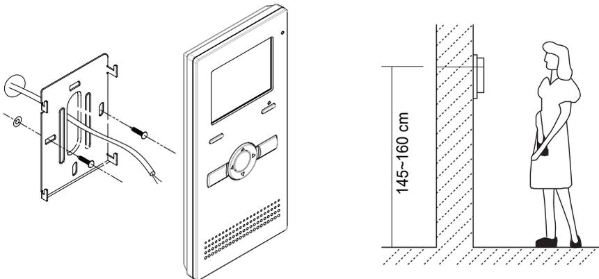
1. Use the screws to fix the Mounting Bracket on the mounting box.(fitting accesories includes a Bracket (Two pieces of 4X25 screws are needed for fastening the Mounting Bracket), Special 2 wire cables to connect with Monitor)
