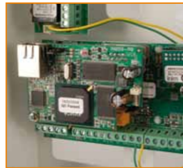
SmartLiving10100L with SmartLAN/G board (particular).
