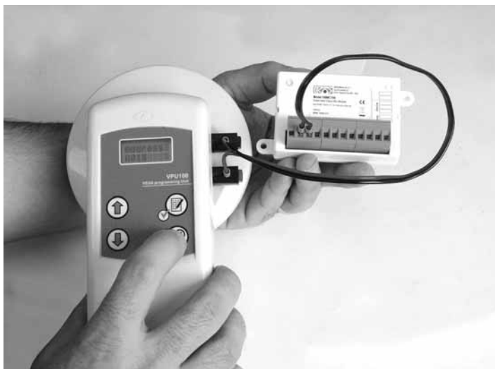
Figure 35 - Addressing modules using a VPU100
