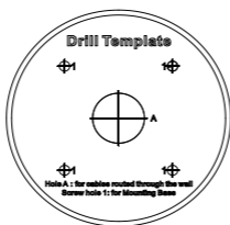
Figure 2-5 Drill Template of the Junction Box
