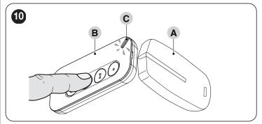
In case of an error, LED (C) will indicate the type of error by flashing:
