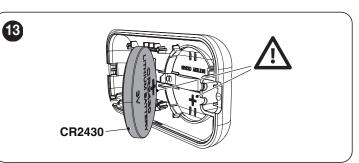
**4.** reassemble the remote control by slotting the protruding parts (3) into their housings (4) and closing the front (C) so that it snaps onto the case (B).
