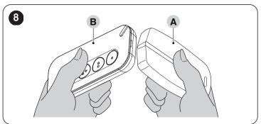
press and hold a button on the reference transmitter (A) until LED (C) of the MYGO lights up
