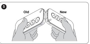
On the NEW transmitter, press and hold any button, within the desired sector, until LED (A) of the OLD transmitter switches on. Subsequently, release the button (LED (A) of the OLD transmitter will start flashing).
