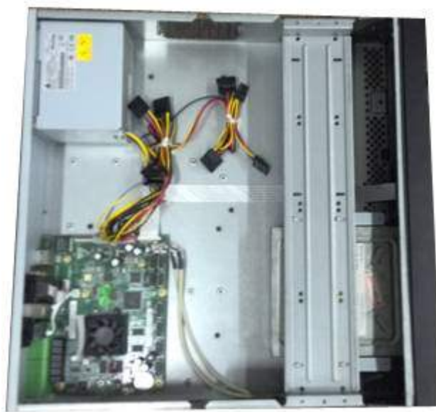
Figure 3-45 Put bracket back
