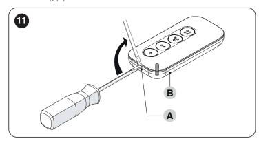
2. press the battery in point (1) and twist the case (B) to release the battery from the clip holding it (2) so that it can be removed
