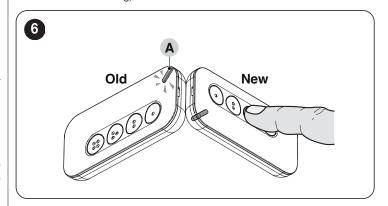
**3.** On the OLD transmitter, press and hold any button, within the desired sector, until LED (**B**) of the NEW transmitter switches on. Subsequently, release the button (LED (**B**) of the NEW transmitter will turn off to signal that the procedure has terminated and the "enabling code" of the NEW transmitter has been transferred).
