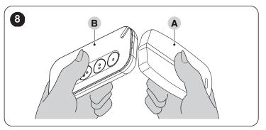
3. press and hold a button on the reference transmitter (A) until LED (C) of the MYGO lights up
