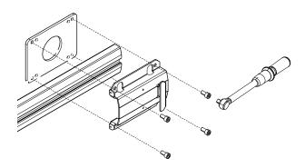
Fix the boom to the anchoring plate.
