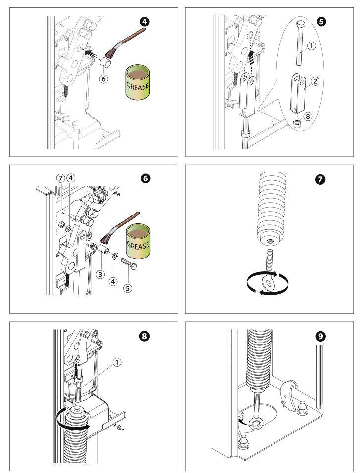
Lubricate the spring when it is fully extended.
