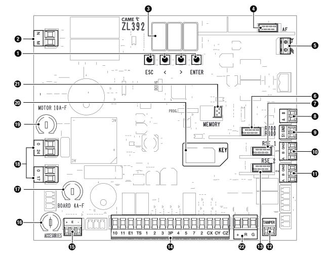
Remove the card cover before inserting the cards into the connectors.
