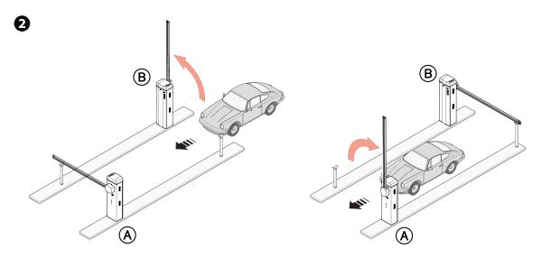
3 OPEN-CLOSE command (2-7) on barrier A or B for emergency opening
