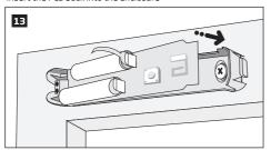
Open the magnet enclosure and screw in (see fig.#16A) or attach the magnet using double-sided adhesive tape (see fig.#16B) to the
