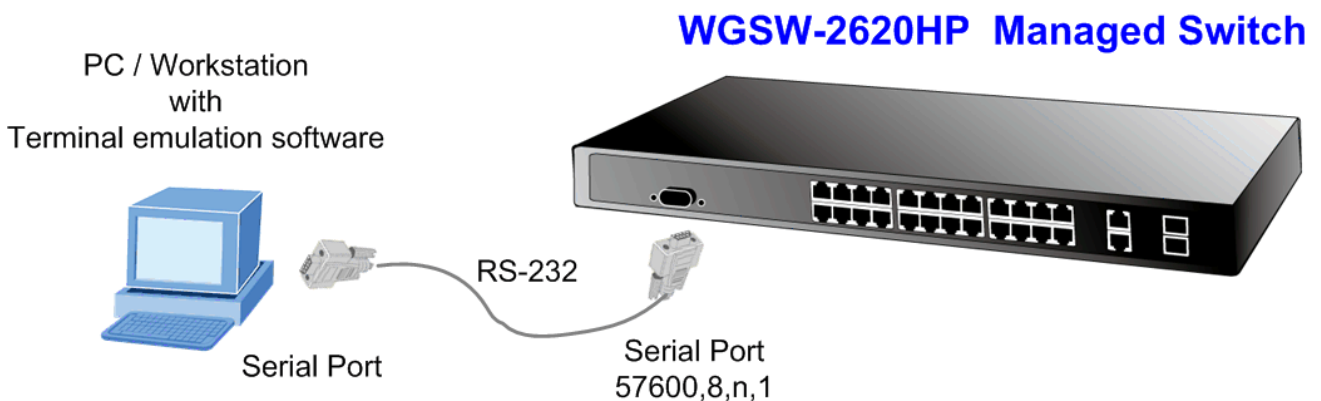
Figure 3-4: Console Management Diagram
